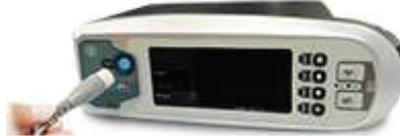
**3** Attach the sensor to the extension as shown below. Use ONLY VPOD ViTAL compatible probes.
